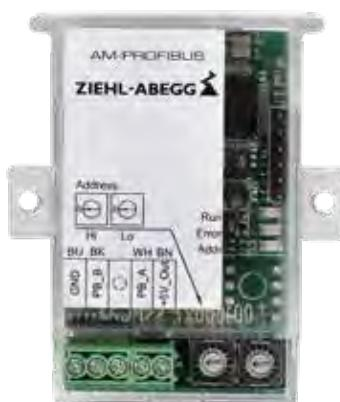
Pluggable add-on modules for function extension of the "Icontrol Basic" and "Fcontrol Basic" without integrated display as well as ECblue motors and fans.
