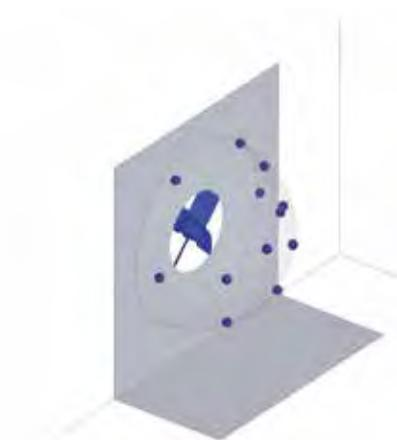
Fig. 1a: Position of microphones
