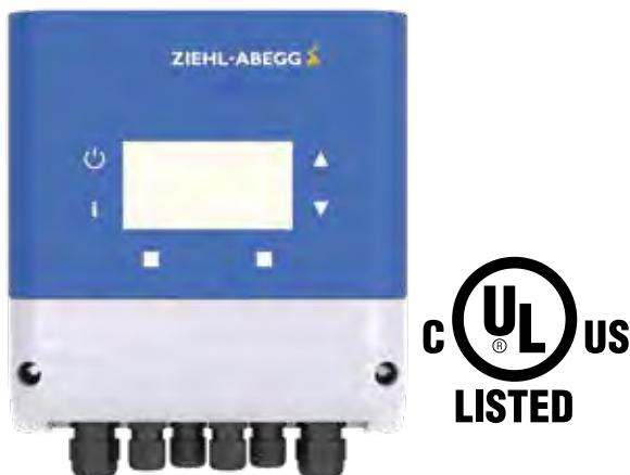
All ZIEHL-ABEGG sensors can be combined with the UNIcon CXE/CXG universal control module. The actual value measured at the sensor is compared with the setpoint. This results in the 0-10 V output signal. Two 0-10 V outputs are integrated. These serve to activate EC fans, frequency inverters and other devices.
