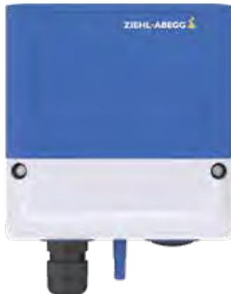
Sensors for measuring differential pressure. Used in air ducts, faninlet nozzles (e.g. in air conditioning box devices), roof fans, etc. The differential pressure sensor is connected to the ventilation system by two pressure connections. The differential pressure thus acts on a silicone membrane, the change in position of which is evaluated electronically.
