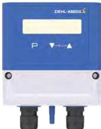
The sensor control module for differential pressure and volume flow measures and indicates the pressure or, optionally, the volume flow in a ventilation system. The calculation of the volume flow is performed by entering the K-factor of the fan inlet ring.
