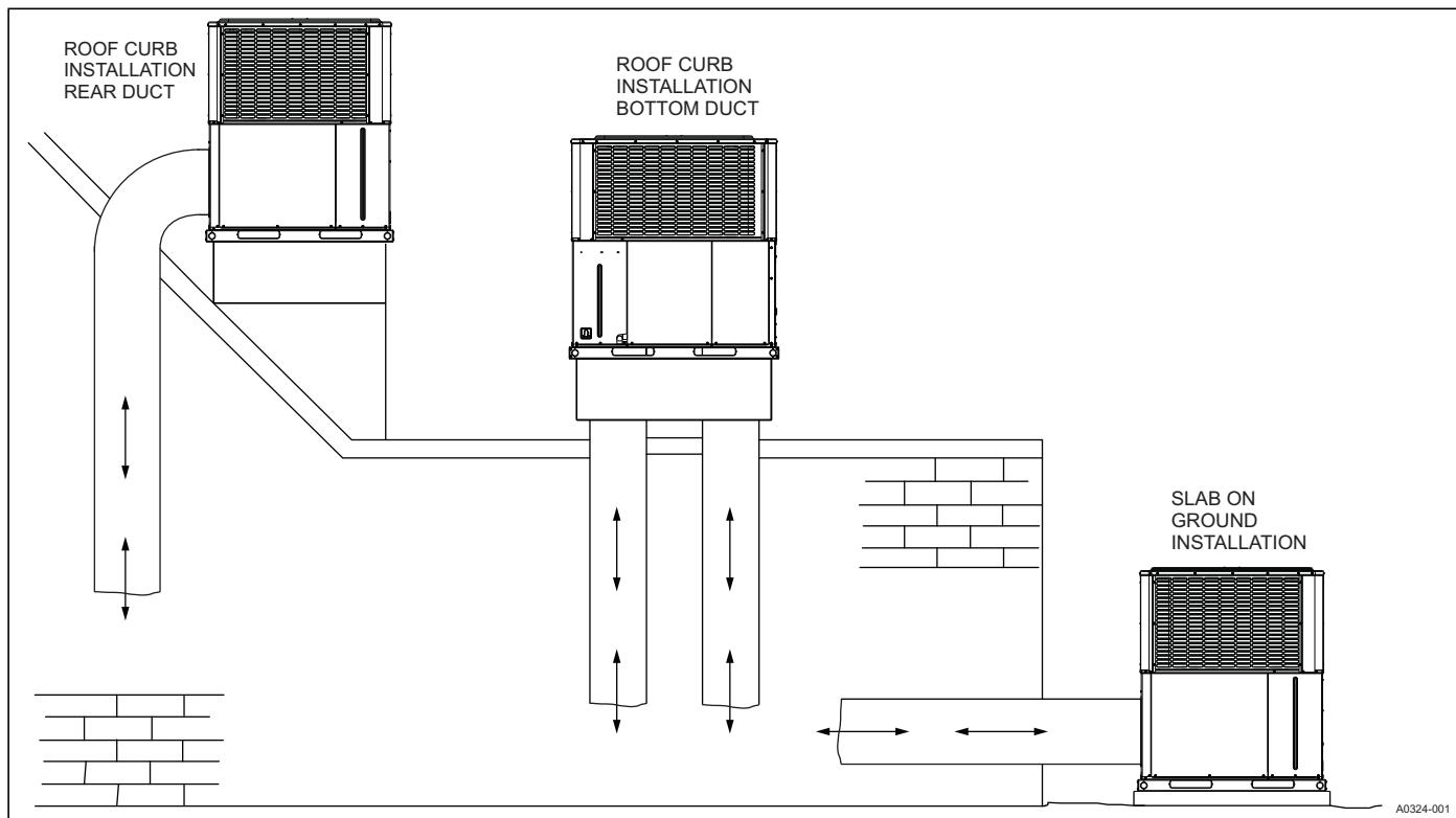
**UNIT TYPICAL SLAB ON GROUND INSTALLATION**
