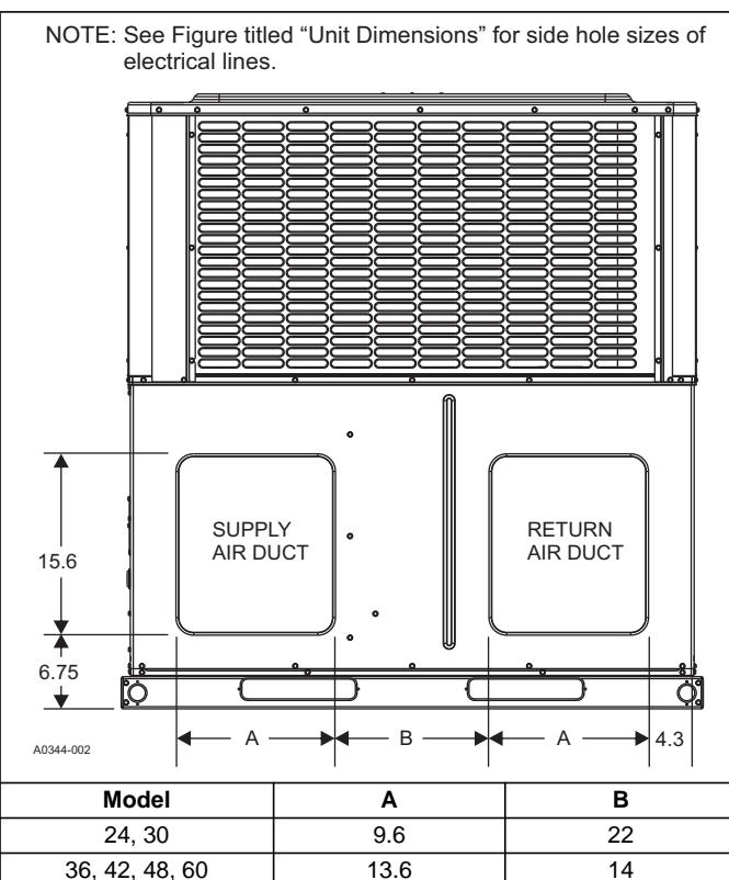
**UNIT TYPICAL DUCT APPLICATIONS**
