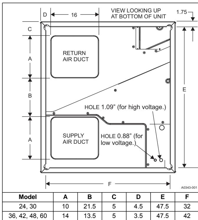
**REAR DUCT DIMENSIONS (Inches)**
