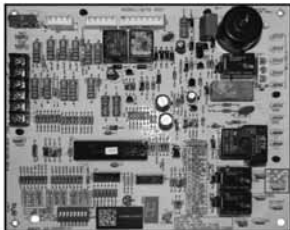
INTEGRATED FURNACE CONTROL
