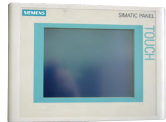
Touch screen controller
