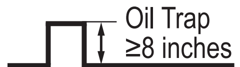
Figure 7: Close Up of An Inverted Oil Trap.
