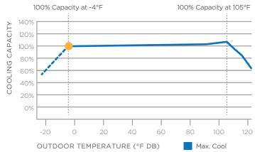
Note: MLA018S4S-1P max cool performance indicated; Data illustrated to -4°F but unit effectively operates to -22°F (indicated by dotted line); 80°F db / 67°F wb entering indoor unit.
