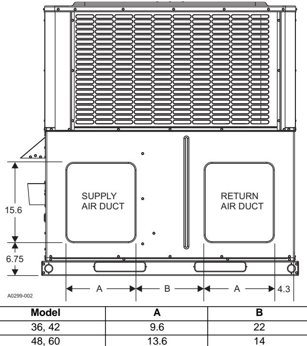
**UNIT TYPICAL DUCT APPLICATIONS**
