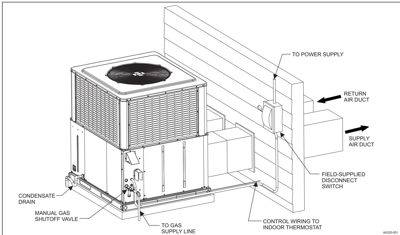
**UNIT TYPICAL ROOF CURB INSTALLATION**
