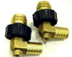
Elbow, 1" Hose Barb X Double O-ring with 1/4" Port and Pressure/Temperature Test Plugs DORB1-90-4HC
