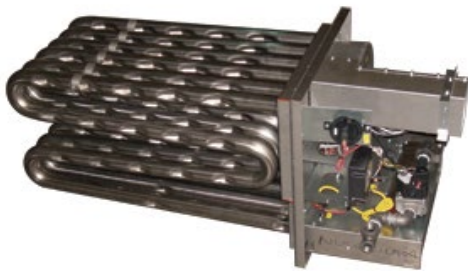
▲ Dimpled heat exchanger provides energy efficient heat transfer and has no internal turbulator, which can corrode over time.
