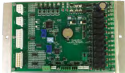
Unit Control Board - Mounted in the AAON Equipment
